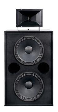
S-2400 speaker system has a passive crossover with cut frequency at 800 Hz, while S-2401 is designed for biamplified applications with external electronic crossover at 800 Hz.
